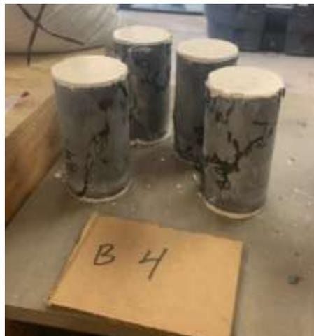
**Fig. 2** 76 mm x 152 mm UHPC cylinders
